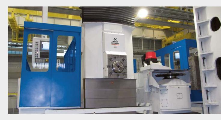
The Innse-Berardi model FCR is a Machining Center for generator rotors. The hydrostatic guideways on all axes, allows to apply high torque and high cutting forces generated during main slots milling by large diameters cutters. Matching on the same carriage the high productivity slotting head with vertical column for auxiliary operations, makes the FCR a versatile center to perform all the machining operations on both generator shaft body and necks.
