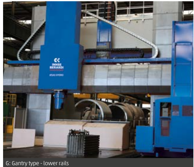
G: Gantry type - lower rails
